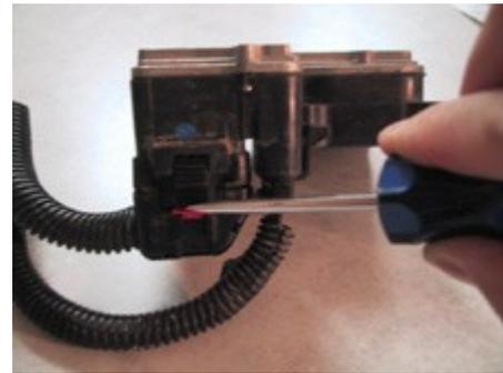
2) Pry the red locking clip into the down position as shown.
