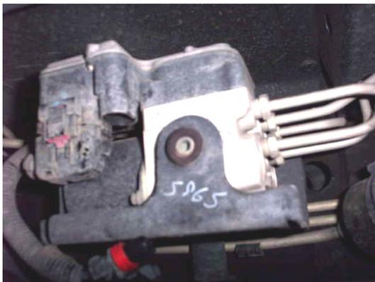
There is very little room to access these four bolts under the truck in such stubborn cases. It is suggested that you disconnect the lines and remove the entire assembly. Take the assembly to a workbench or drill press to drill/grind the heads off of the bolts. If this sounds too ugly and disconnecting the five brake lines will ruin your day; you can instead remove the three hex head bolts attaching the ABS pump/manifold to the vehicle frame and CAREFULLY lower it. You must
