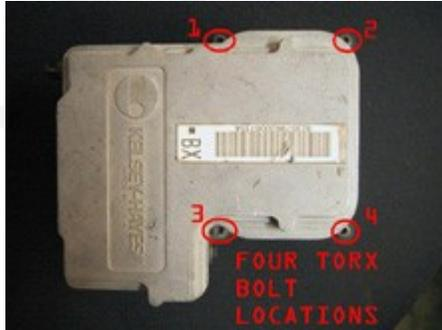
Be sure to order a bolt replacement Kit to replace rusted or stripped out Torx ABS module bolts.
