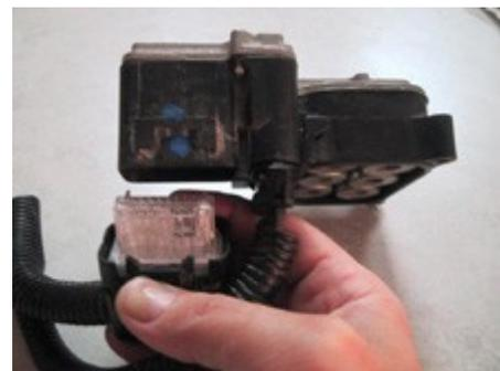
support the heavy pump assembly so you don't kink the brake lines. Then you will have room to get a small grinder or Dremel Tool to grind the heads off of the evil rusted bolts.
